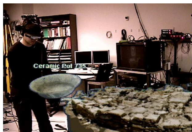
Figure 8. Our augmented reality visualization system. A user in our lab explores a full-size model of the site and selects one of the findings to examine in detail.
