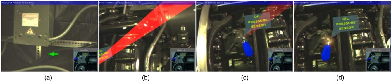
Figure 2: A typical localization sequence in our prototype. (a) A screen-fixed arrow indicates the shortest rotation distance to target. (b) As the user orients on the target, a semi-transparent 3D arrow points to the target. (c) When the user orients on the target, the 3D arrow begins a gradual fade to full transparency. (d) When the arrow has completely faded, a brief highlighting effect marks the precise target location.
