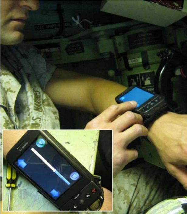
Figure 3: A mechanic uses the wrist-worn controller to cue the next task in a repair sequence. The inset view shows additional features that appear during applicable tasks for controlling animations.
