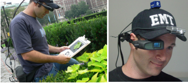
Figure 6: Head-worn display, video camera, and orientation tracker mounted on baseball cap.
